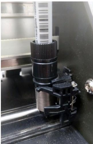
Next, take the pen out of the holder and place it into the clip on the right of the machine. Do this while the machine is off. Ensure that the pen is located EXACTLY as in the image to the left, with the top channel fitting into the semicircular holder and the spring clip grabbing onto the lower channel.
